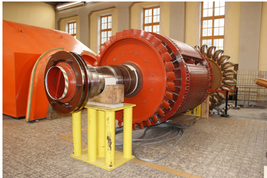
(b) 36 MVA Pelton wheel generator (source: Wikimedia Commons , Asurnipal, CC BY-SA 4.0)
