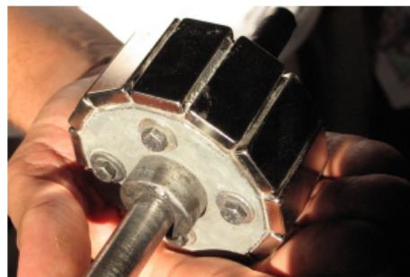
Fig. 2.18: PMs on a rotor (source: flickr.com, AIDG, CC BY-NC-SA 2.0)
