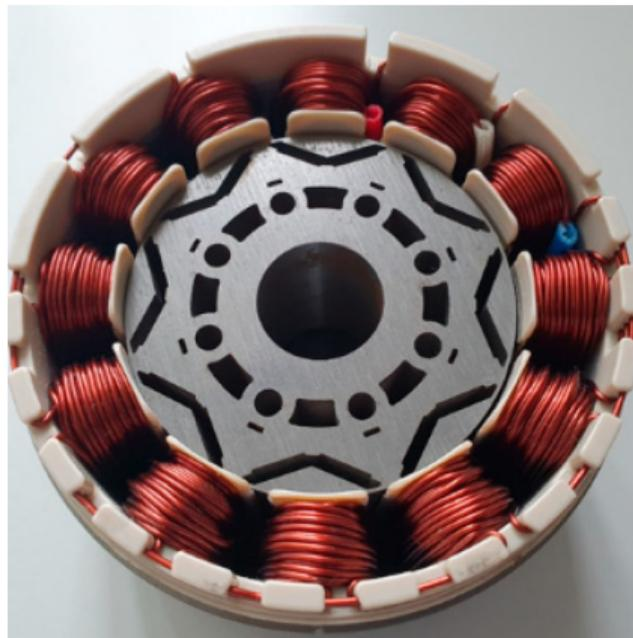
Fig. 5.16: Example of a concentrated winding where conductors form coils centered around single stator teeth (source: Chan-Ho Baek et al., *Iron Loss Analysis of a Concentrated Winding Type Interior Permanent Magnet Synchronous Motor with Single and Dual Layer Magnet Shape*, MDPI Machines, 2021, [CC BY 4.0](#))
