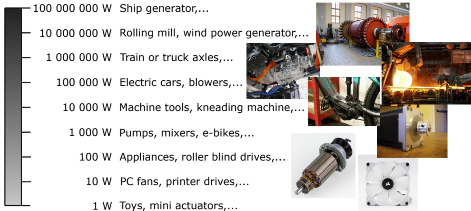
Fig. 1.9: Power range overview (inspired from A. Binder, *Elektrische Maschinen und Antriebe* (lecture slides), Darmstadt University, 2022 with additional figure sources: [A. Wolf](#), [Asurnipal](#), [M. Williams](#), [R. Spekking](#), [Foxcorner](#), [A. Tredz](#) and [J. Halicki](#) under varying CC licenses)
