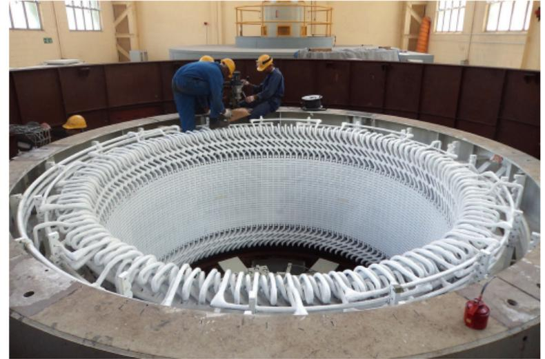
(b) Hydrogenerator with form-found stator winding
