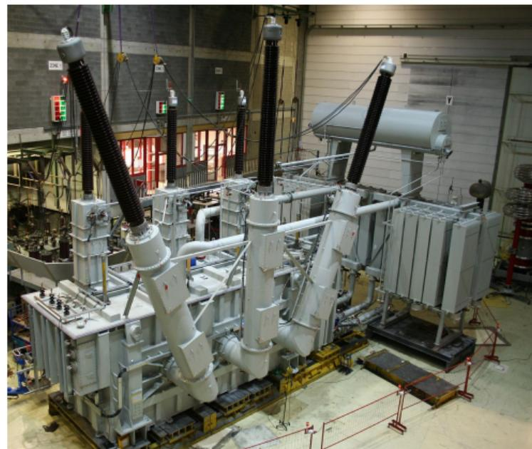
Fig. 4.22: 750 MVA, 380 kV / 230 kV three-phase autotransformer (source: [Wikimedia Commons](#), P. Mertens, CC BY-SA 3.0)
